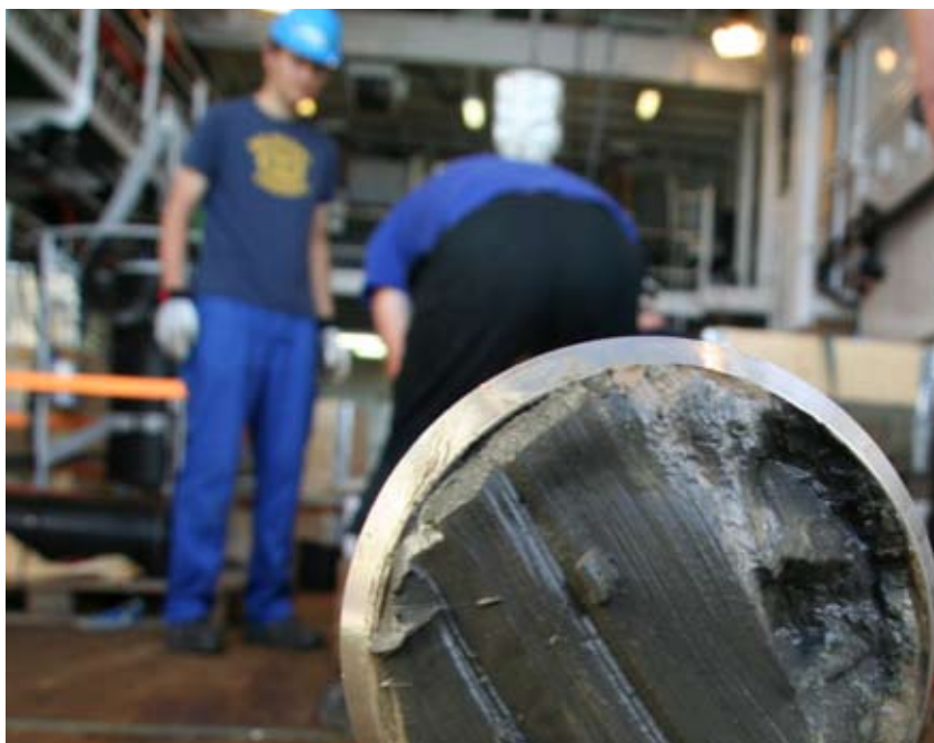
A gravity core can collect up to four meters of sediments (photo: Jill Johannessen, BCCR).
