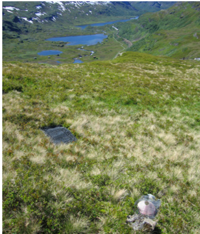
● Pollen and macrofossil traps at Upsete that have collected pollen and plant remains since 2004. Traps are emptied every autumn and their contents are analysed to show annual variation in production and deposition of fossils from different plants near the present day tree line. PHOTO: ANNE BJUNE
